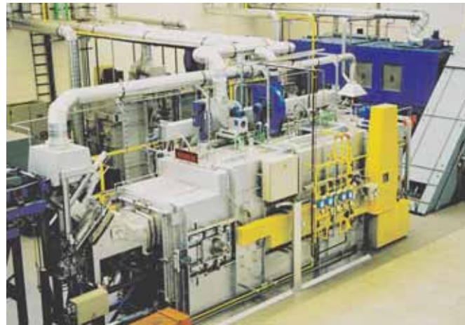
Fig. 1: Partial view on a hardening and tempering line with a nominal throughput of 2000 kg/h
