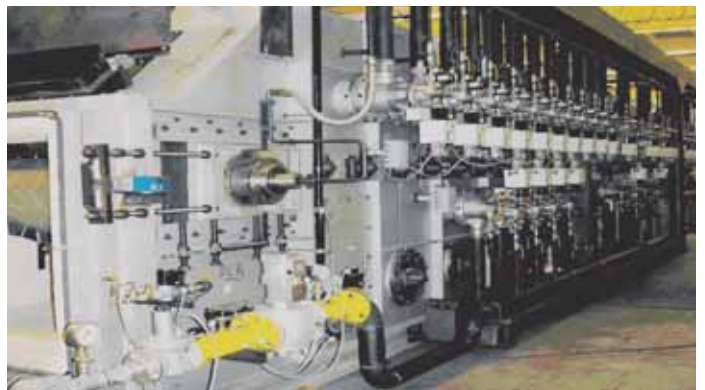
Fig. 2: Cast link belt furnace for a production rate of 3000 kg/h with opened maintenance front door
